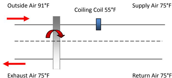
Alternative 3 includes adjusted load distribution when using a 0.80 efficient enthalpy wheel. Energy savings is now even better combining the new solar shade design and incorporating an enthalpy wheel in the new variable air volume air handling unit. Here is the new and improved load distribution.
